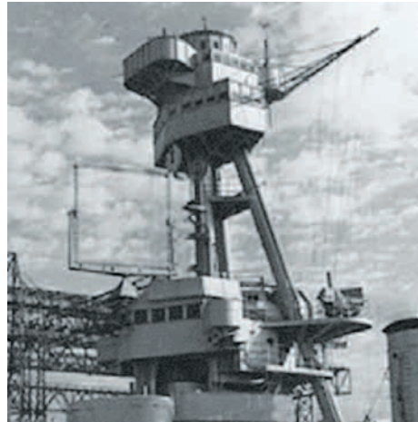
The XAF radar system on the USS New York. This was the first operational US radar, and it was invented, developed, and installed by the NRL. (Photo courtesy of NRL)
